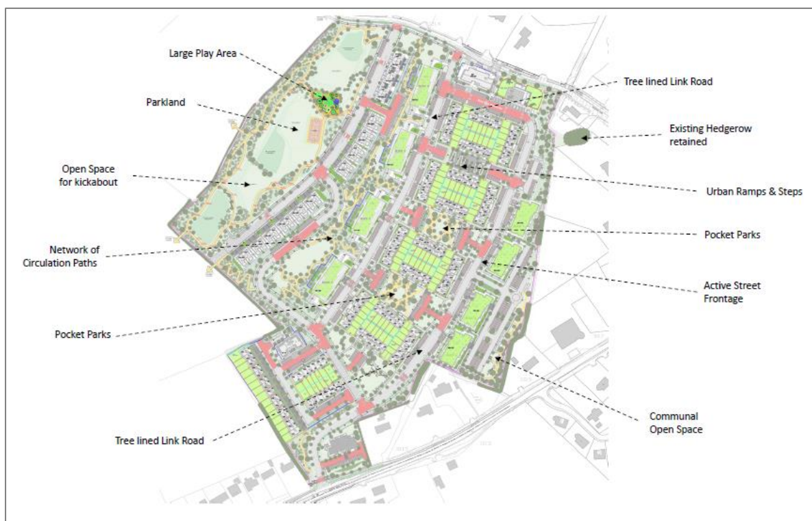
Figure 2-7. Hierarchy of Green Open Spaces throughout the Scheme (source: RMDA Landscape Architects)
